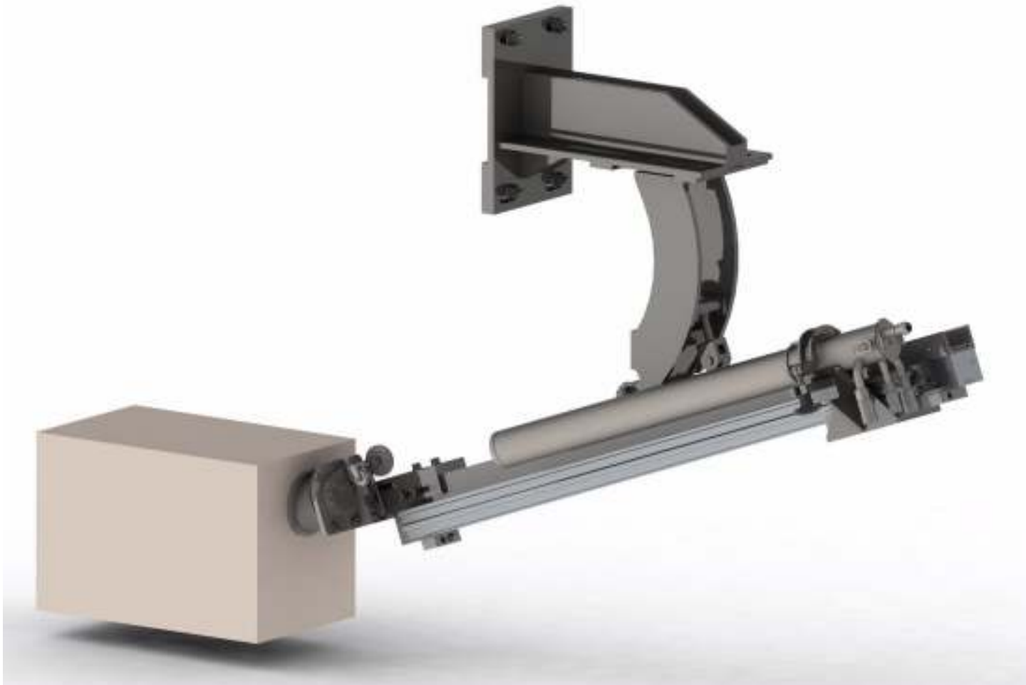
Picture 1a: GS New Furnace camera system
